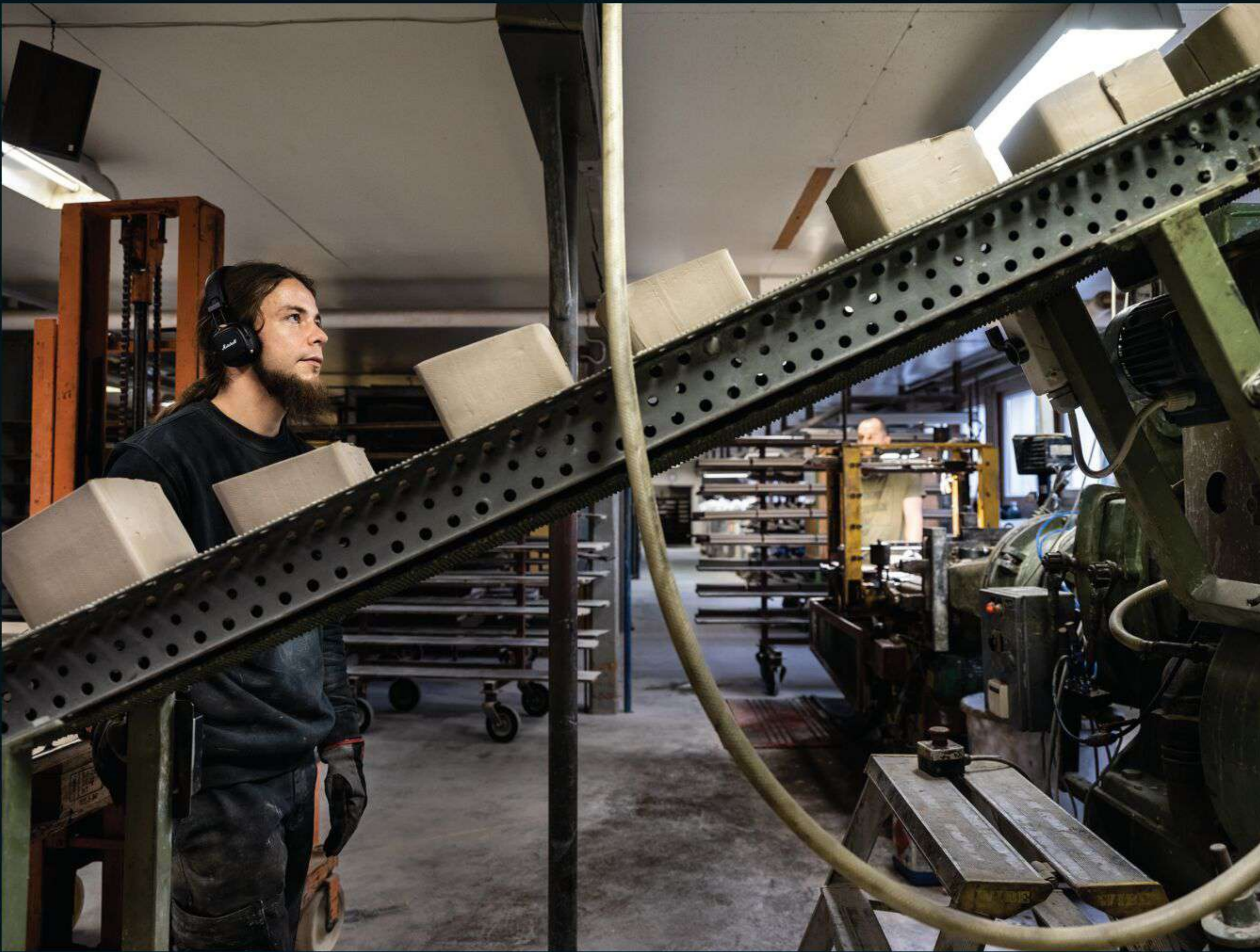
Blocks of clay are moved into the tile extrusion machine in one of the first stages of the production process. The clay is produced from powder that's partly made from recycled ceramics.
