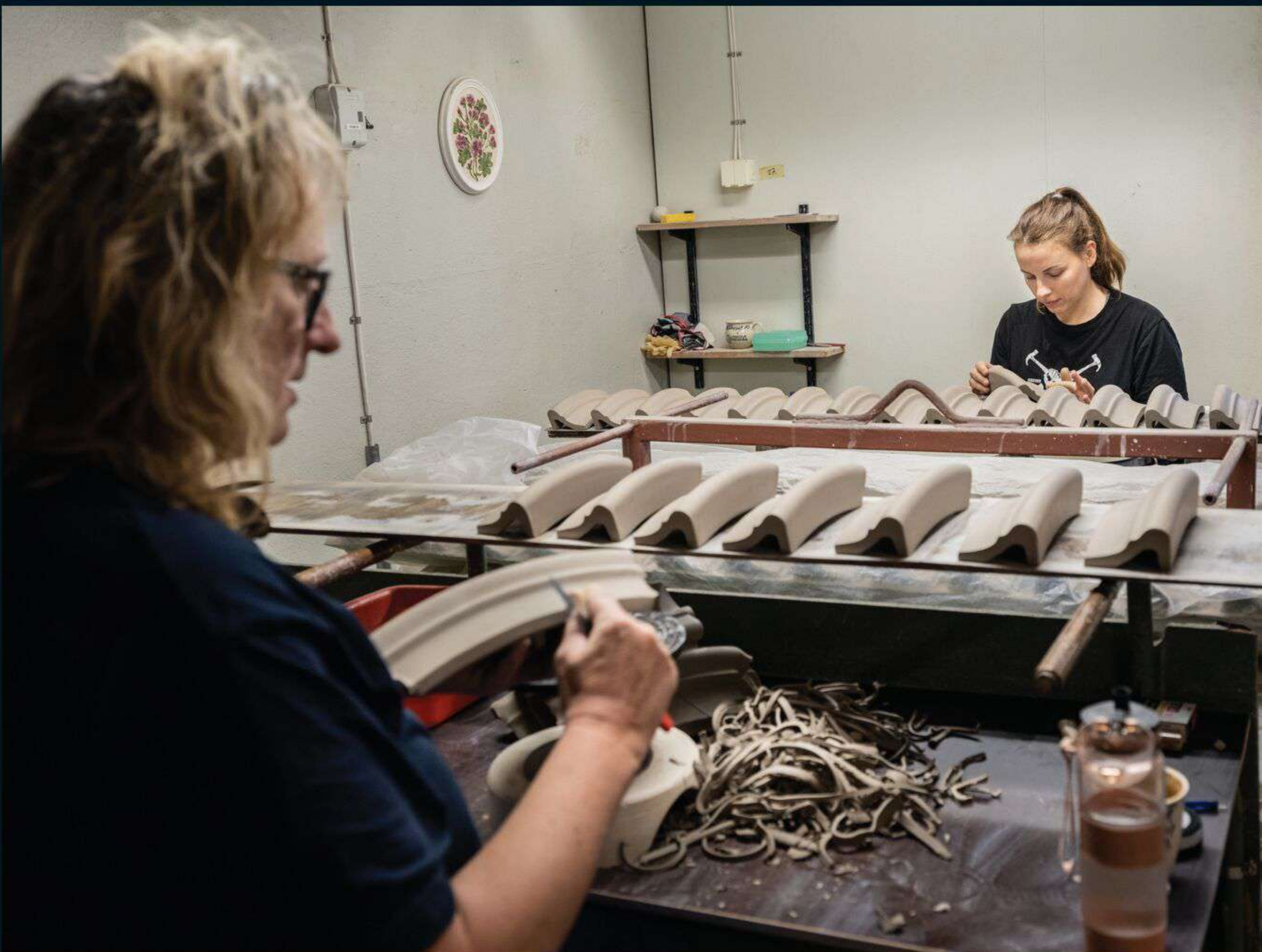
Two workers polish the surface of tiles that are normally used to decorate the outside of the stoves. A standard version of a stove contains more than 80 individual pieces, all crafted by specialists.
