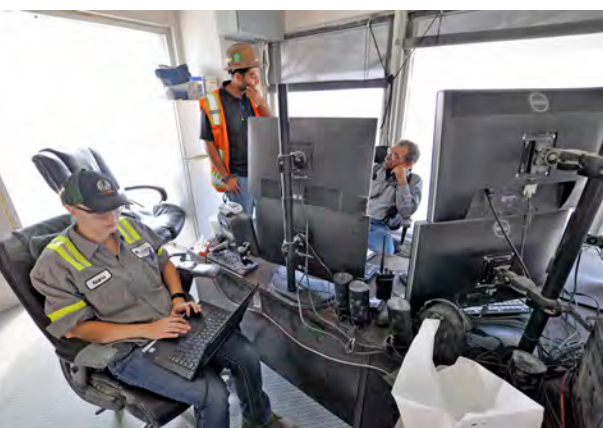
Metallurgist I Alaina Mallard, senior metallurgist Rahul Singh, and mill operator II Floyd (George) Mocaby discuss the expert system inside the ore crusher's control room.
